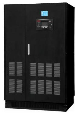
MU8000LF33 UPS 80 ~ 500 kVA provide maximum protection and power quality for mission critical loads, including data centers, industrial processes, telecommunications, security and electro–medical systems. It is an on–line double conversion UPS with IGBT–based 3–level PWM rectifier technology, featured with high input power factor (> 0.99), low THDi, high efficiency (maix. ≥ 94%) and built–in output isolation transformer.
